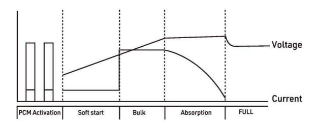
**PCM Activation:** Once the charger has been properly connected to the battery it will deliver a constant pulse frequency to activate the PCM before it enters into the charge program
